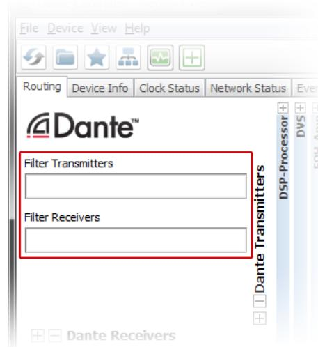
The filtering is case-insensitive. For example, in the Dante Controller Network view [shown here](#), entering the string “foh” in either of the Filter fields would display only the FOH-Amp and FOH-Console devices, and their channels.
