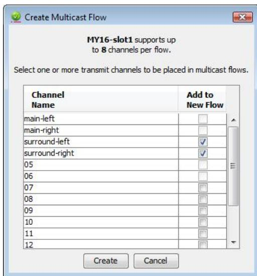
The window shows a list of the Tx channels for the device, and allows you to add them to the new multicast flow that is being created, by checking the tick box next to each channel name. Once you have selected all the channels required, create the multicast flow by clicking the **Create** button at the bottom of the dialog box. To abandon creating a new multicast flow, click **Cancel**.
