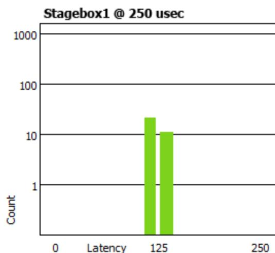
If any bars are amber, it means that some packets are arriving near the limit of the latency setting. Network traffic fluctuations could potentially lead to extra delay which could cause packets to arrive late. A histogram of this type indicates that the receiver latency should be increased if possible.
