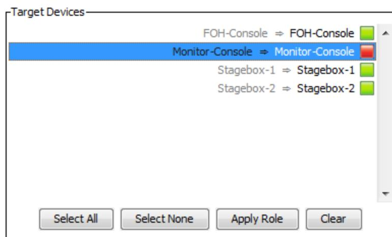
The LED icons against each device indicate the assignment status of the device.
