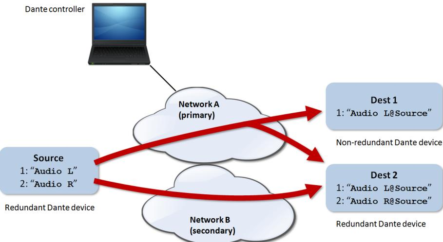
If the secondary network is connected to a device that supports redundancy, it is enabled automatically. The same audio data is transmitted on both the primary and secondary networks simultaneously. In the event of a failure on one network, audio will continue to flow via the other network.
