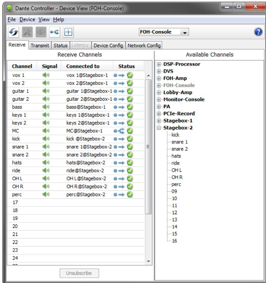
The label of the device being viewed is displayed in the middle of the toolbar. In the screenshot above, FOH-Console is the device being displayed in the drop-down list box.
