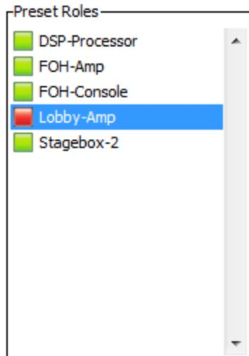
You can apply a role to the same physical device from which it was created (if it exists in the target network), or to a different device in the same network, or to another device in a new network.
