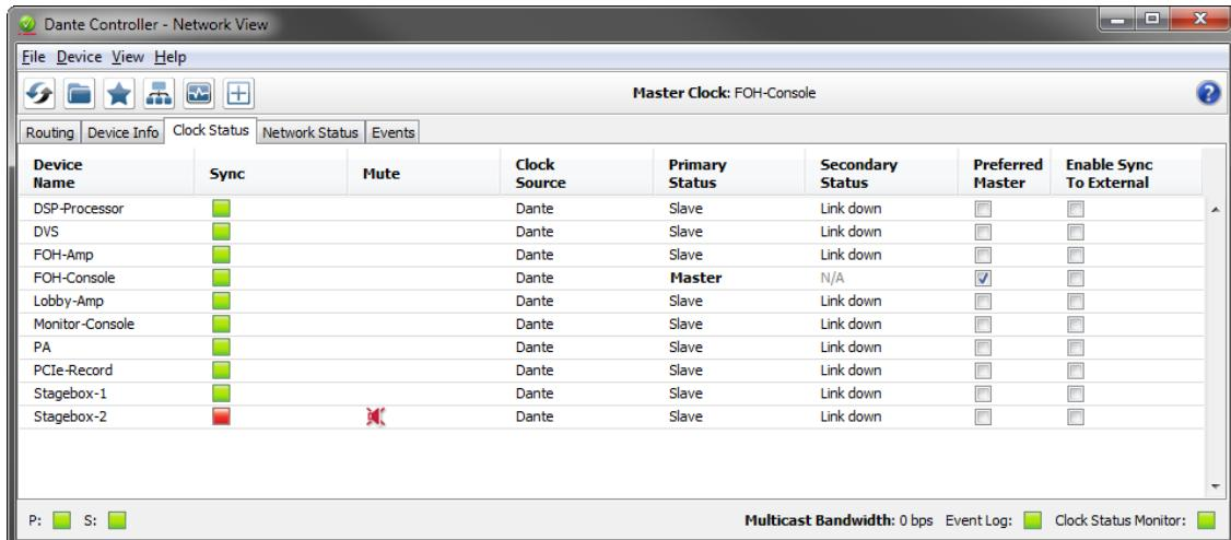
The screenshot shows the Dante Controller software interface with the 'Clock Status' tab selected. The table displays the following data:
