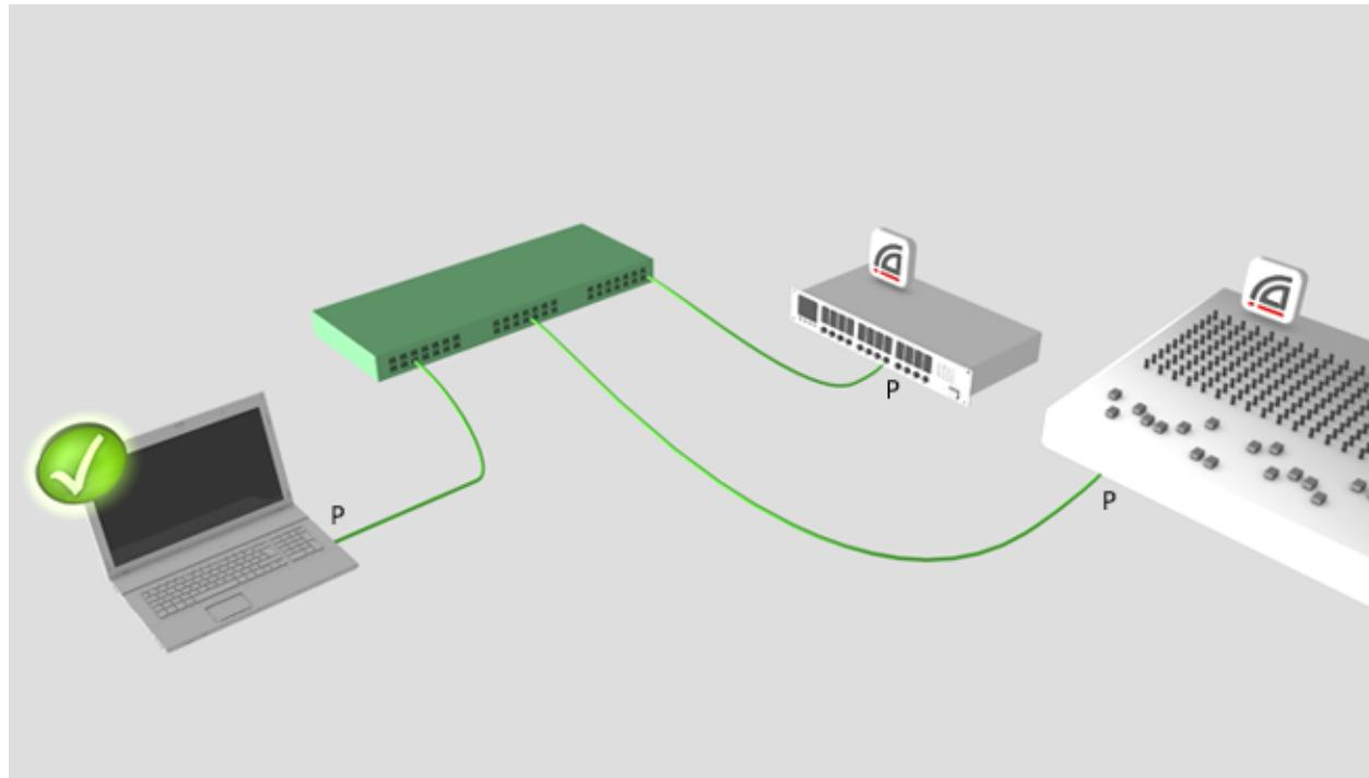
**Primary and secondary Dante networks (redundant configuration), only one network interface on the host computer**
