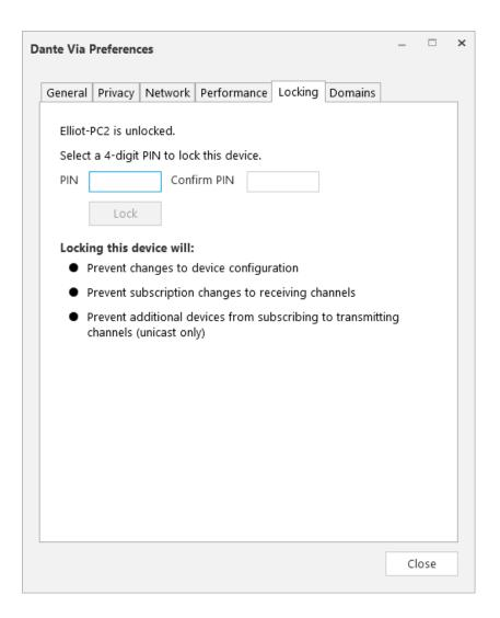
Use the Locking tab to lock and unlock Dante Via.
